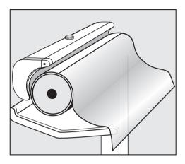
Completely unwind the padding cover attached to the roller and let it hang down smoothly.
